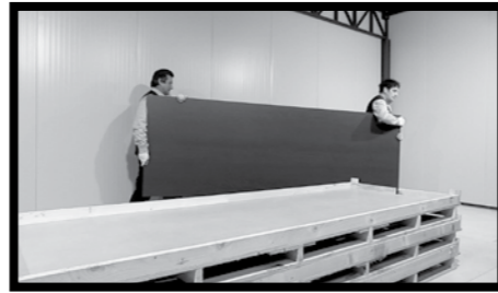
Fig.3 - When the slab is upright, hold it from its top edge and shift it keeping it straight and upright. This operation should be performed with the aid of a second person.
