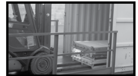
Fig.8 - To take on pallets from their short side (e.g. when unloading containers), you must use forks with a length of at least 2.5 metres to guarantee a sufficiently long supporting surface and therefore protection of the package and its contents.
