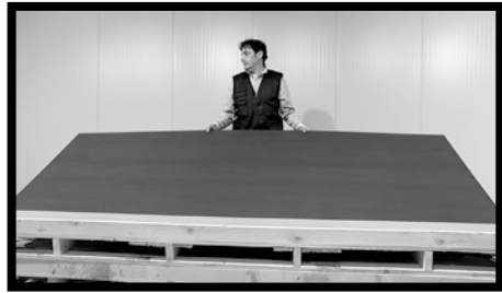
Fig.1 - 300x100 cm slabs of KERLITE and KERLITE PLUS can be lifted by one person only. Lift the slab with open hands. Slowly raise the longer side so as to eliminate the suction effect, due to contact with the underlying slab, and ensure a good grip.
