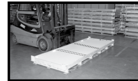
Fig.7 - To take on pallets from their long side, position the forks at a distance of at least 1 metre the one from the other, perpendicular to the long side of the pallet and at the centre of the latter. Forks must be supporting the entire surface of the pallet.
